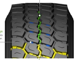
**Tie Bars Design**Tie bars between each block prevents irregular wear.
