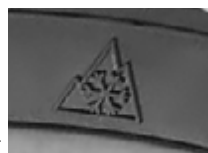
Complies with international standard tire conditions and has high snow performance, allowing direct driving even when restricted by tire chains in winter. The tires are engraved with the three-peak Mountain snowflake logo and M+S.
